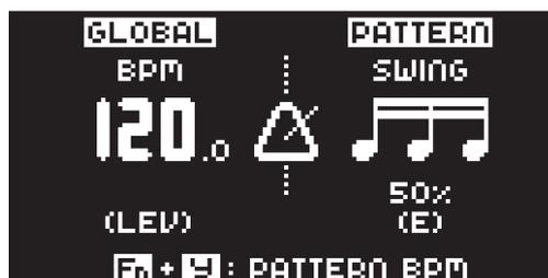
Turn **DATA ENTRY** knob **E** to set the SWING ratio to 51-80%. The default setting is equal spacing, 50%.
