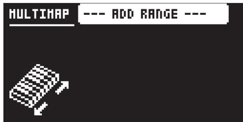
**RANGES** are the basic building blocks of the multi map. They define what function that is assigned to each key or key range. A multi map can contain up to 128 ranges. The ranges can be set within the note interval C0–G10. If no ranges exist, select ADD RANGE.
