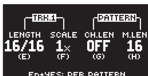
The TRACK column sets the step length and scale of the track. The settings only affects the active track. Press the **[TRK]** keys to select the track whose scale settings you wish to edit.
