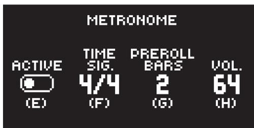
**ACTIVE** activates/deactivates the metronome. You can also press [FUNC] + [PTN] and hold for a second to toggle the metronome on and off when you are not in the METRONOME menu.
