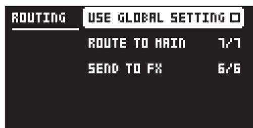
**USE GLOBAL SETTING** uses, when ticked, the global audio routing settings for the active pattern.
