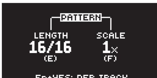
**LENGTH** controls the step length of the pattern. The leftmost number displays the number of steps in the pattern. The total length, displayed by the second number, determines the maximum number of steps available in the pattern. If you use 17 steps or more in a pattern, the [PAGE] key is (while in GRID RECORDING mode) used to toggle between the different pattern pages.
