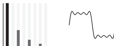
The additive method can be used to make many different timbres. This combination of partials, for example, sounds close to a bell tone.
