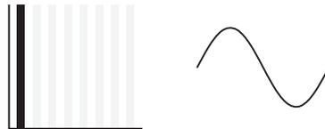
Adding every partial in series will replicate a sawtooth. Note how the volume decreases for each partial, creating a natural falloff.
