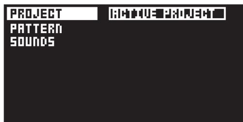
The column to the left selects what will be backed up. Select the column using the [LEFT] arrow key. Use the [UP]/[DOWN] keys or the **TRACK LEVEL** knob to navigate in the column. The SysEx data send alternatives located in the column to the right will change depending on the selection made in the left column. Press the [RIGHT] arrow key to access this column. Use the [UP]/[DOWN] keys or the **TRACK LEVEL** knob to select what will be sent. Press [YES] to initiate the SysEx send procedure.
