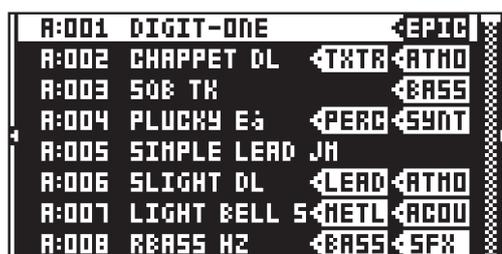
Press [LEFT] to access the SORTING menu. Press [YES] to execute the commands. Press [NO] or the [RIGHT] arrow key to exit the menu.
