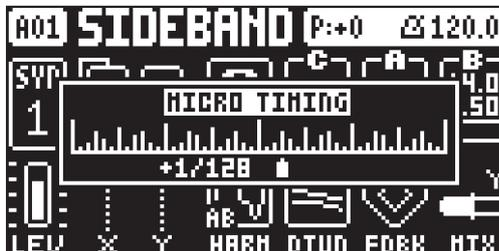
**MICRO TIMING** Press [LEFT]/[RIGHT] keys to adjust the time offset.
