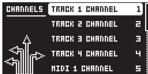
**TRACK 1–4 CHANNEL** selects dedicated MIDI track channel that controls the synth tracks. It also sets the MIDI channel for the MIDI messages the *DATA ENTRY* knobs on the chosen track send. An OFF setting makes the track disregard any incoming MIDI messages.
