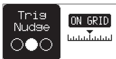
1. In GRID RECORDING mode, press and hold one or several [TRIG] keys and then turn SWING to access the TRIG NUDGE menu that shows the time offset for the chosen sequencer trig(s) on the active track.
