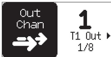
**T1-6 OUT** selects the dedicated MIDI channel that is used to send (by turning the knobs) parameter data from a specific track. If configured as OFF, parameter data are not sent via MIDI.
