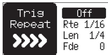
**ON/OFF** Toggles the retrigger function ON/OFF for the chosen trig.
