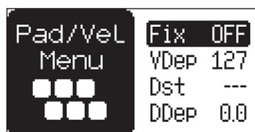
**FIX** Pad velocity set the pads to trig with a fixed velocity, and sets the value of the fixed velocity. OFF sets the pads to respond to dynamic velocity. (1–127, OFF)
