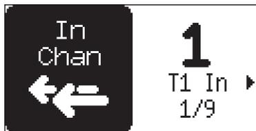
**T1-6 IN** selects the dedicated MIDI channel that is used to receive parameter data to a specific track. If configured as OFF, parameter data are not received via MIDI.
