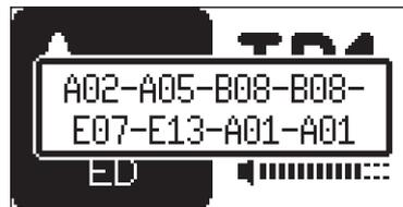
You can create one chain, and it can contain any pattern in bank A–H. The chain can consist of up to 64 patterns.
