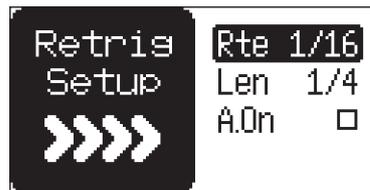
**RTE** Sets the retrigger rate (1/1, 1/2, 1/3, 1/4, 1/5, 1/6, 1/8, 1/10, 1/12, 1/16, 1/20, 1/24, 1/32, 1/40, 1/48, 1/64 or 1/80). 1/16 is the nominal retrigger rate, one trig per step. 1/32 corresponds to two trigs per step and so on. To trig triplets, for example, set the retrigger rate to 1/12 (or 1/24).
