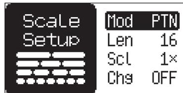
**MOD** Mode can be set to either PATTERN or TRACK. In PATTERN mode all tracks share the same SCALE and LENGTH settings. In TRACK mode, all tracks can have individual SCALE and LENGTH settings. Press [T1-6] to select the track to set the scale for.
