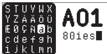
In the NAMING menu, turn the **LEVEL/DATA** knob to navigate between the character positions. Press and hold **[FUNC]**, and then turn the **LEVEL/DATA** knob to select a character for the highlighted position.
