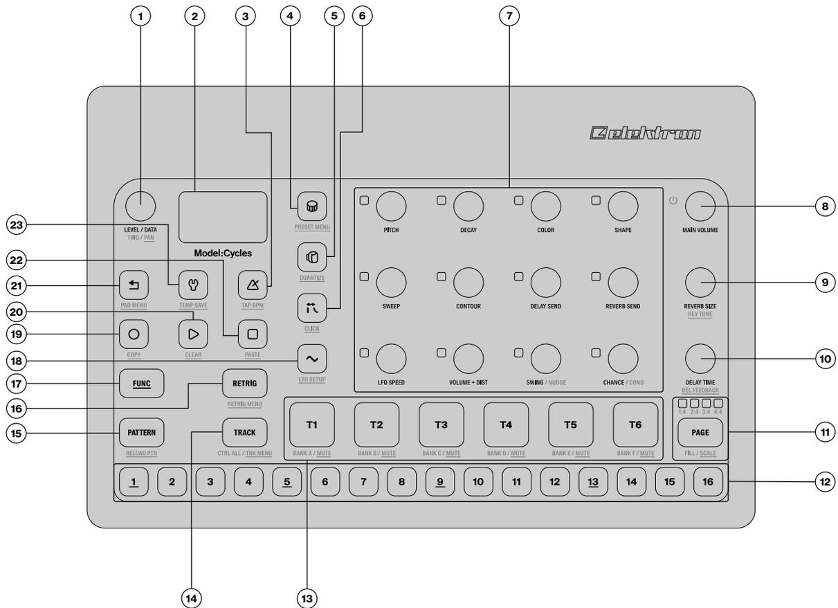
1. **LEVEL/DATA** sets the overall volume level of the active track. You also use it to set parameters and navigating menus. The secondary function sets the track pan.
